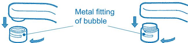
Turn the accessory of external and internal thread with coin and attach the Branch faucet tightening cap on the faucet.
